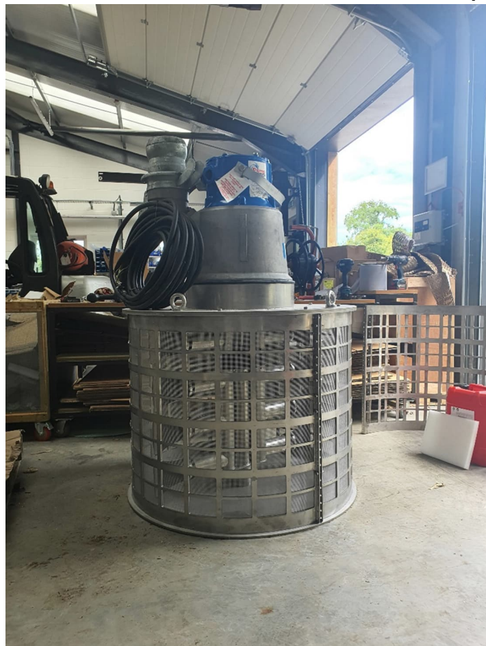
Figure 3-5- Rotorflush RF800LW Based Strainer Pump Unit
